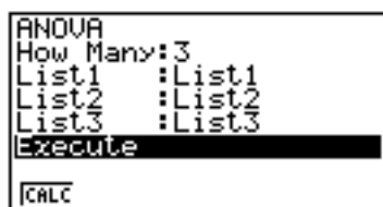
Figure 1: Setting up a one-way analysis of variance on a Casio cfx-9850G Plus
