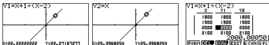
Figure 18: Exploring the asymptotic behaviour of f(x) = x + 1/(x - 2) .
